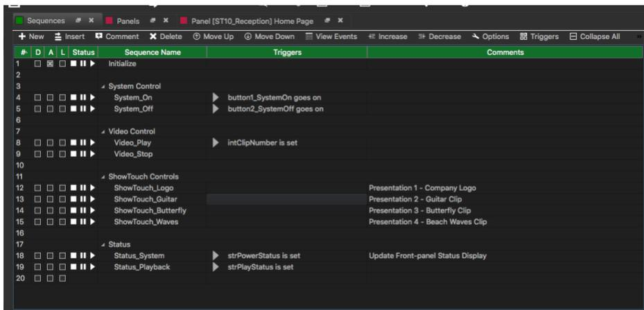
The script starts off with an 'Initialize' Sequence which does nothing more than initialize the front-panel display of the V16X. This clears the display and writes some text on the screen that says "LED Wall Example".
