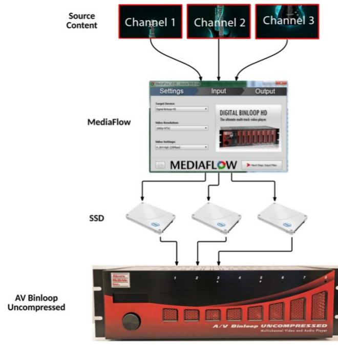
The quickest and easiest way to load content to the SSD drives is by interfacing to them directly from a computer using a SATA adapter. A USB 3.0 SATA adapter is included with every AV Binloop Uncompressed for this purpose.
